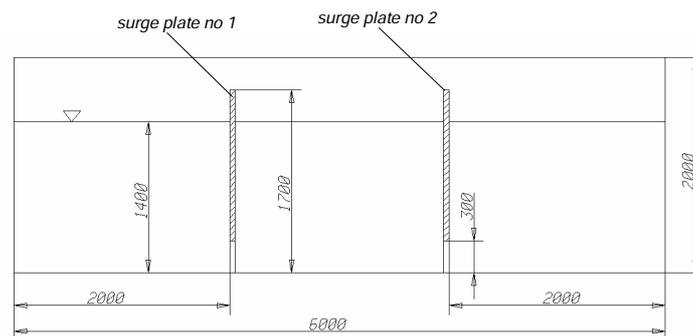
Fig. 2. Dimensions of tank that was used in CFD simulation
