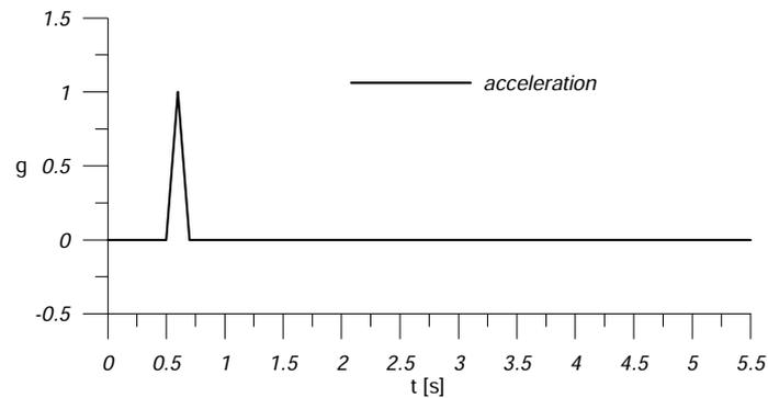
Fig. 4. Acceleration acting on the tank
