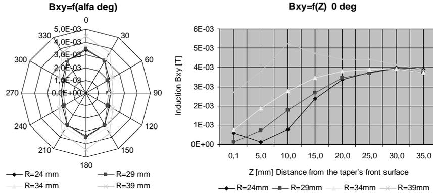
Fig. 7. Radial component of magnetic induction (measured by the sensor) in the plane parallel to rope axis and in the function of distance from the taper's front surface
