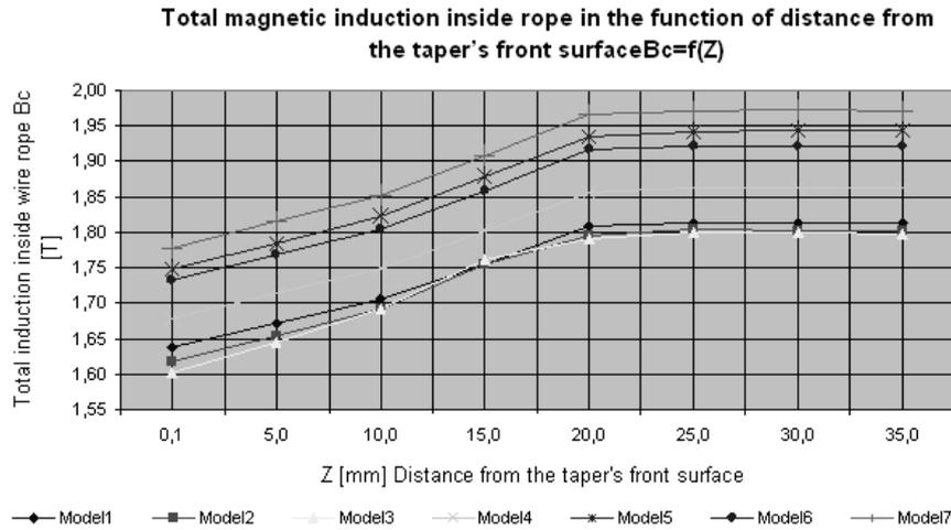
Fig. 8. Magnetic induction in the rope in all considered variants of the analysis
