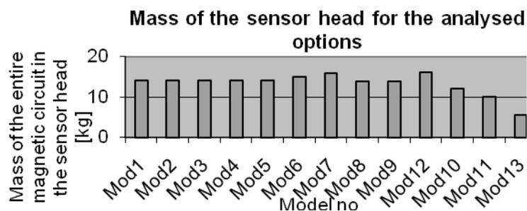
Fig. 5. Mass of the device for particular options of decision variables
