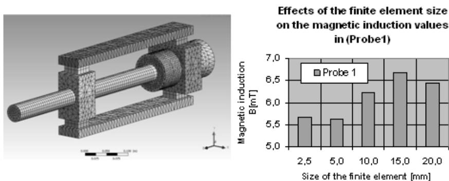
Fig. 4. Discrete model and the influence of the finite element size on measurement data at the given measurement point
