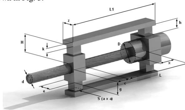
Fig. 3. Decision variables for optimization of the magnetic circuit
