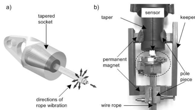
Fig. 1. a) Rope attachment in a socket – model, b) Magnetic sensor head placed on the rope attachment point (tapered section)
