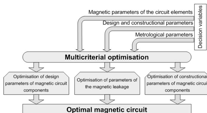
Fig. 2. Multi-criteria optimization of a magnetic circuit
