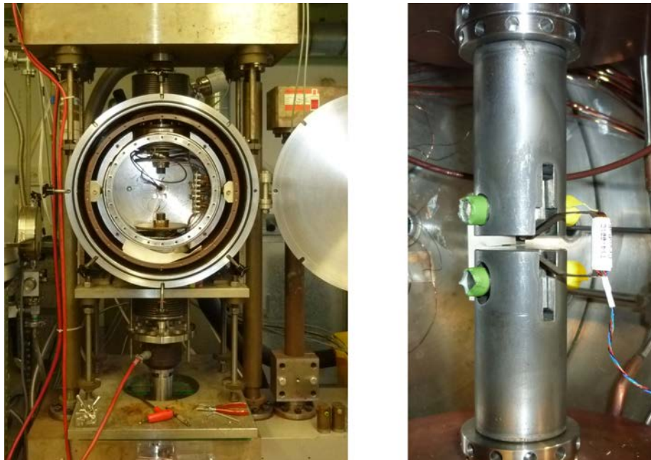
Figure 4.22.: Cryogenic mechanical testing facility at KIT [85] (left) and specimen mounted by means of special grips and with on purpose designed extensometer (right).
