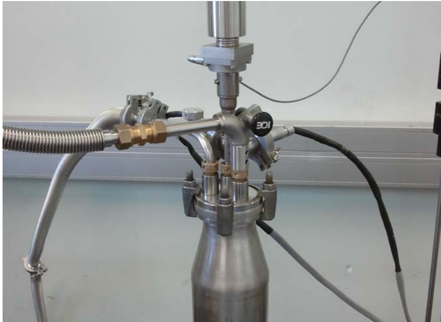
Figure 4.9.: Helium inlet and outlet as well as signal connectors.
