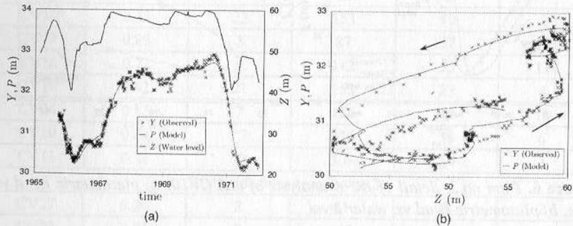
Figure 8. Dam no.1, IRFA analysis of P1 piezometer during the exploitation phase: a) piezometric head vs. time, b) piezometric head vs. water level
