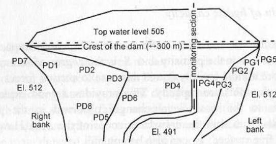
Figure 9. Dam no.3, map showing the location of piezometers at the dam site
