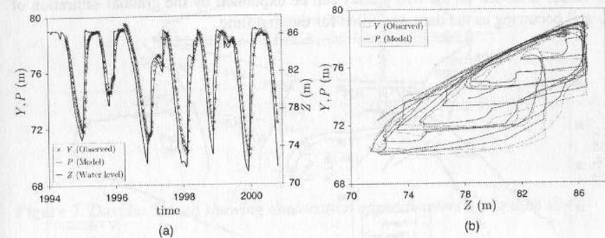
**Figure 5.** Dam no.2, IRFA analysis of cell CV10: a) piezometric head vs. time, b) piezometric head vs. water level
