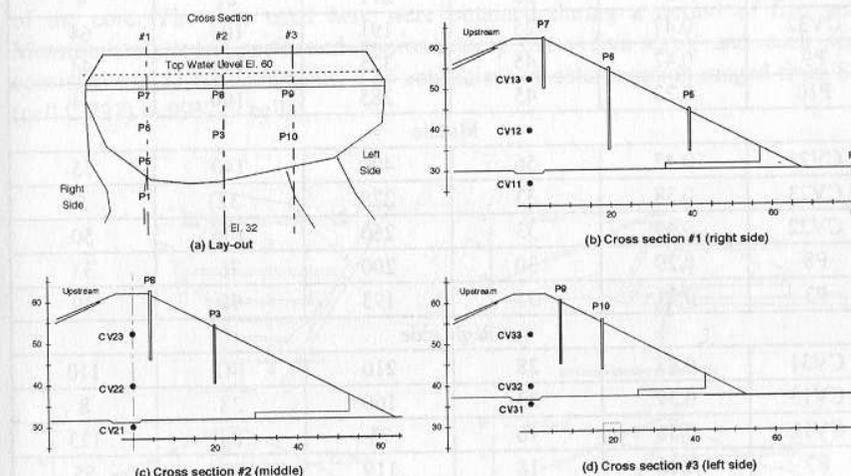
**Figure 3.** Dam no.1, lay-out, cross-section locations, piezometer and pore-pressure cell locations
