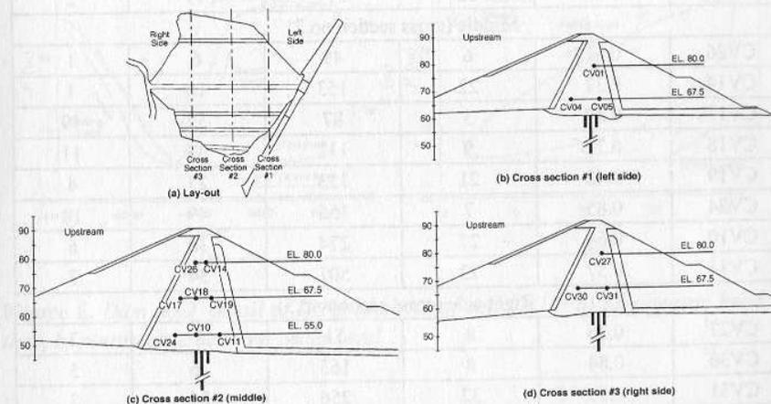
Figure 4. Dam no.2, lay-out, cross-sections and pore-pressure cell locations
