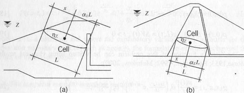
**Figure 2.** Interpretation of parameters  $\alpha_z$  (relative distance from the measurement point to the drainage system),  $\eta_z$  (characteristic response time of the measurement point) and  $L$  (mean length of the seepage path): a) homogeneous earthdam, b) zoned earthdam
