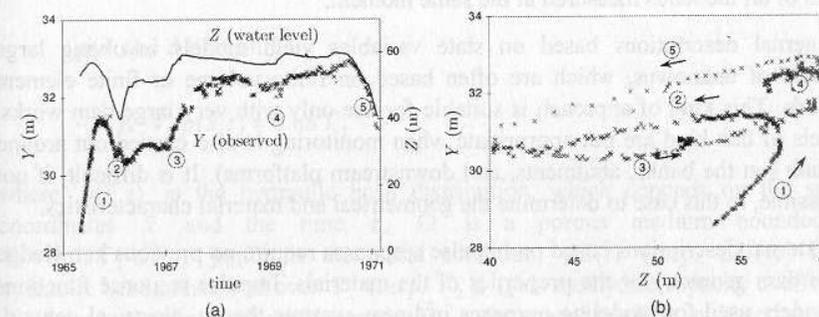
**Figure 1.** Example of piezometer data: a) piezometric head vs. time, b) piezometric head vs. water level and hysteresis of a cyclic rise/drop in the water level
