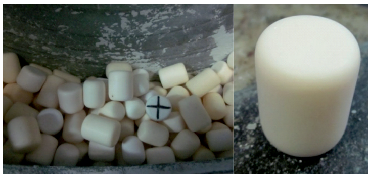
Fig. 2. Grinding bodies – cylinders of material VC-100-2
