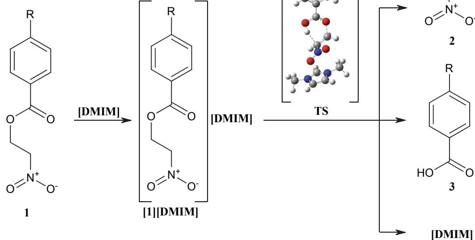
**Scheme 1.** Mechanism of the decomposition reaction of nitroethyl benzoates catalyzed by the 1,3-dimethylimidazolium cation
