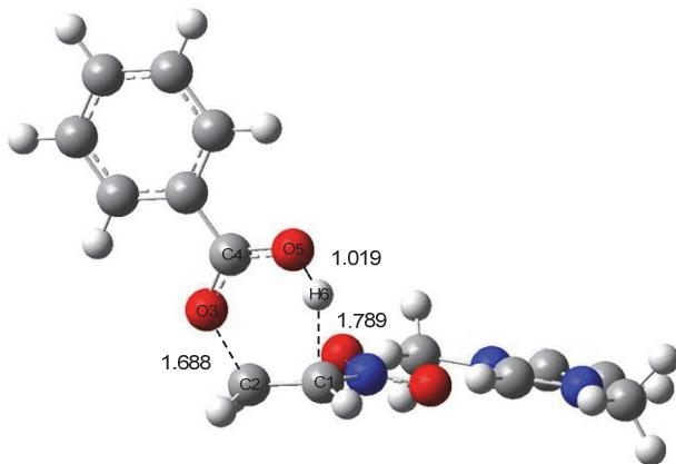
**Fig. 3.** Transition state TS structure for the decomposition of nitroethyl benzoates **1a** catalyzed by the DMIM cation
