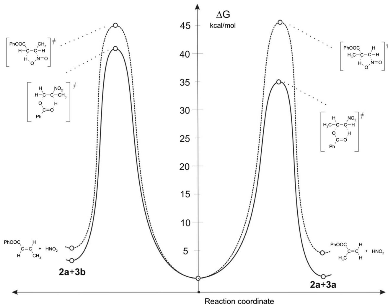
**Fig. 1** Gibbs free energy profiles for thermal decomposition of esters 1a and b in gas phase according to B3LYP/6-31G(d) calculations (T=298 K)
