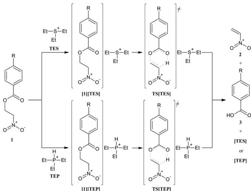
**Scheme 1.** Mechanism of the decomposition reaction of nitroethyl benzoates catalyzed by the triethylsulfonium (TES) and the triethylphosphonium (TEP) cations.
