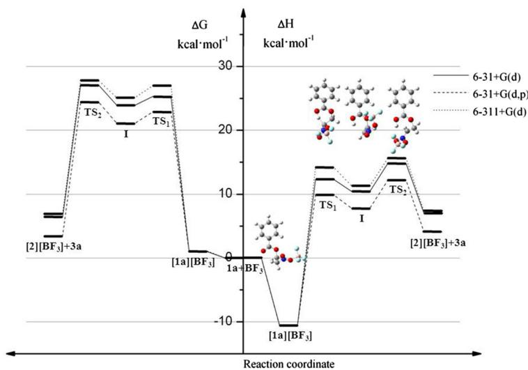
**Fig. 4** M06-2X/6-31 + G(d) enthalpy and Gibbs free energy profiles for decomposition of nitroethyl benzoate **1a** catalyzed by  $\text{BF}_3$
