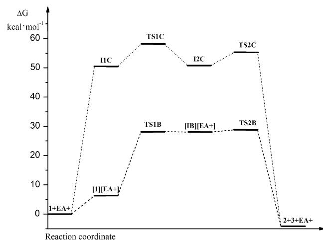
**Fig. 1.** Energy profiles for decomposition of nitroethyl benzoate **1** catalyzed by (EA<sup>+</sup>) according to data of B3LYP/6-31+G(d, p) calculations.
