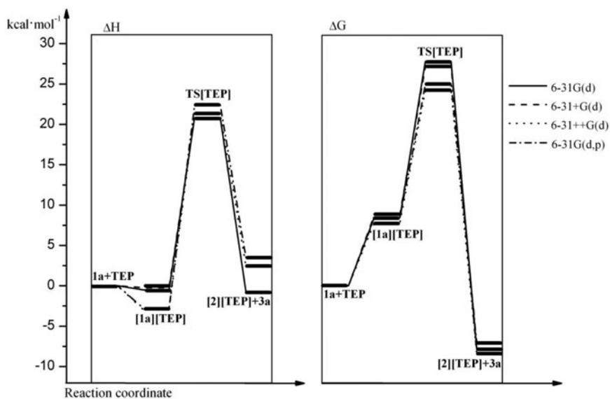
**Figure 2.** Energy profiles for the decomposition of nitroethyl benzoate **1a** catalyzed by the triethylphosphonium cation.
