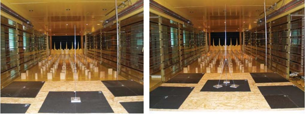
Fig. 4. Models of the masts: cantilevered (a) and tripod (b) in the wind tunnel working section
