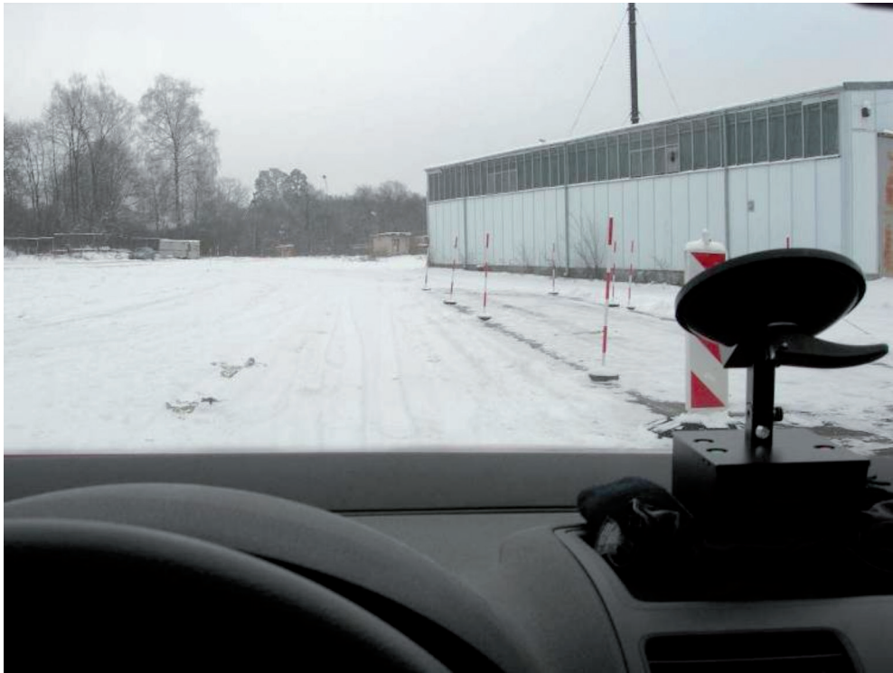
Fig. 2. The experimental road sector with a snow-covered asphalt-concrete pavement (the accelerometer installed in the car)
