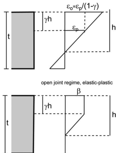
Fig. 2 A simple one-dimensional elastic-plastic "opening joint" model
