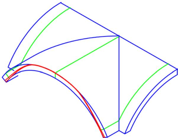
Fig. 21 The cross vault with Sabouret cracks
