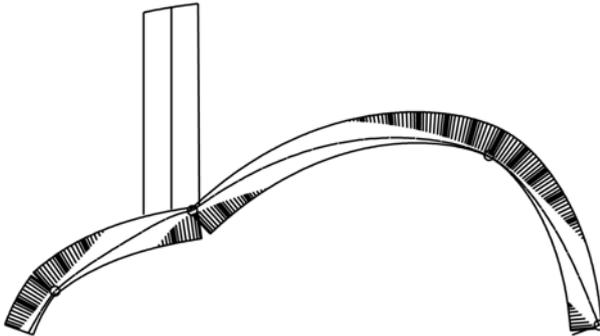
Fig. 14 Arch under the action of an additional load. Formation of the fourth hinge (scale factor 200)
