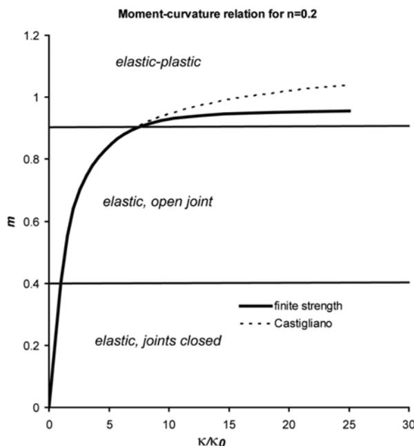
Fig. 3 Moment-curvature relation for an elastic-perfectly plastic “opening joint” model
