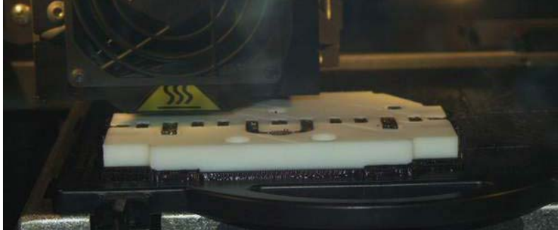
Fig. 5. Generation of control valve body by means of Rapid Prototyping method
