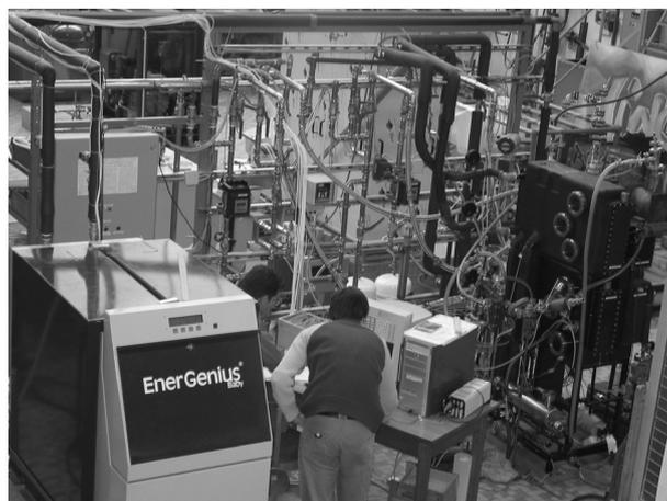
Fig. 2. Test facility at TUB with 10 kW chiller (right) and cogeneration engine (left)
