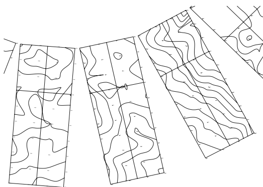
Fig. 8. Plate deformation isolines upon tensioning [4]
