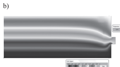
III. 6. a) Connection detail of window sill and external wall, b) Temperature distribution in the analyzed node – Therm
