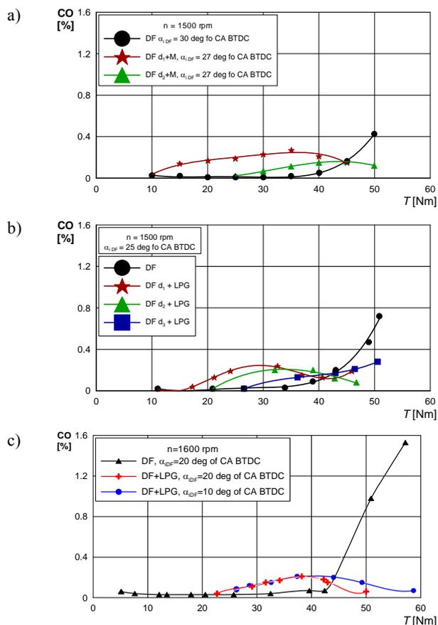
Fig. 3. Comparison of CO emissions for fuelling modes: a), b) and c) (described in chapter 1)
