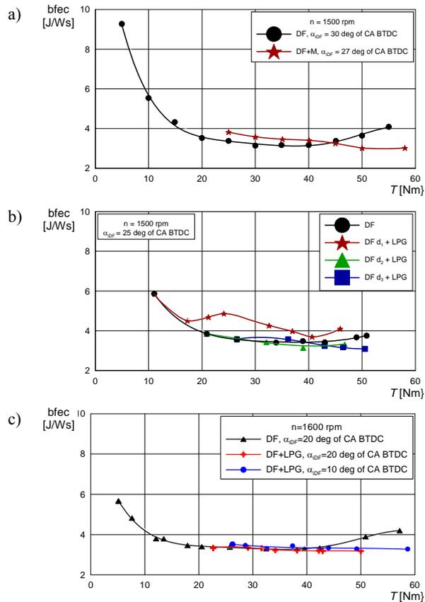
Fig. 2. Comparison of load characteristics of specific energy consumption for fuelling modes: a), b), and c) (described in chapter 1)
