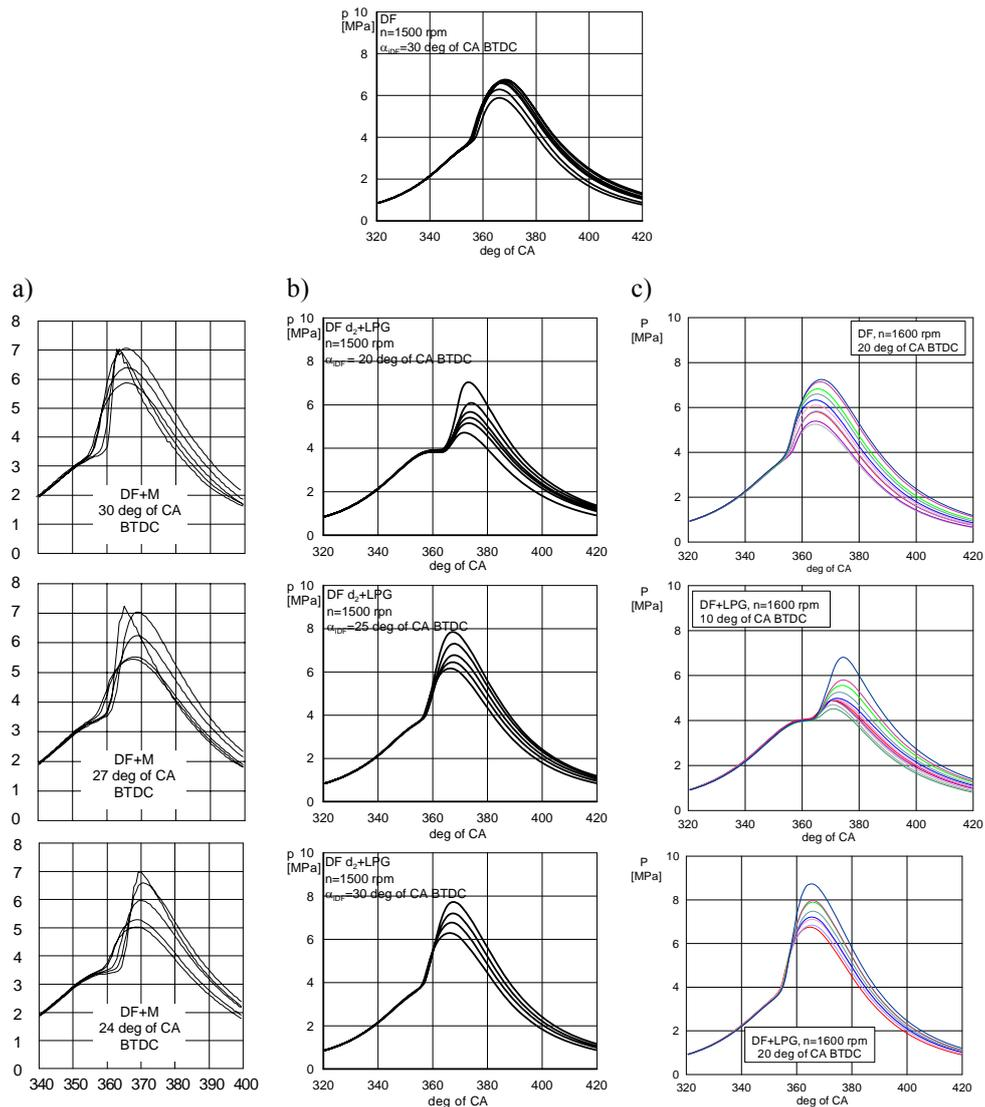
Fig. 7. Combustion pressure versus crankshaft angle  $P=f(\alpha)$  for the standard fuelling (with diesel oil only) and for fuelling modes: a), b) and c) (described in chapter 1)
