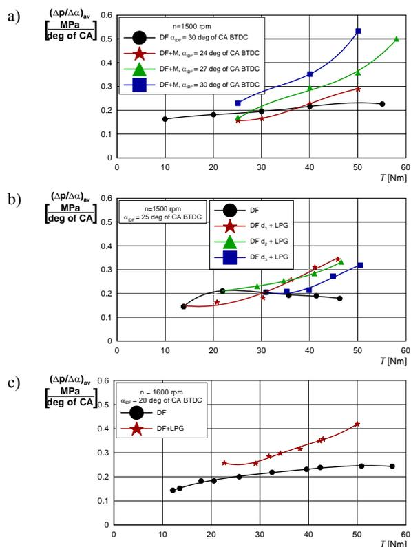
Fig. 9. Variability characteristics of average rate of pressure rise  $(\Delta P/\Delta \alpha)_{av}$  for various injection timings of the pilot fuel and for fuelling modes: a), b) and c) (described in chapter 1)
