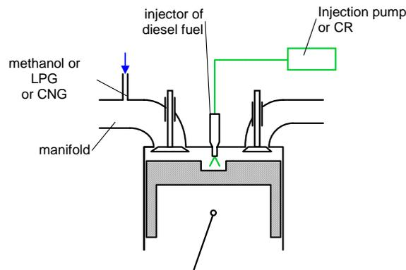
Fig. 1. Overall scheme of dual fuelling of a compression ignition engine where the main fuel is methanol or LPG
