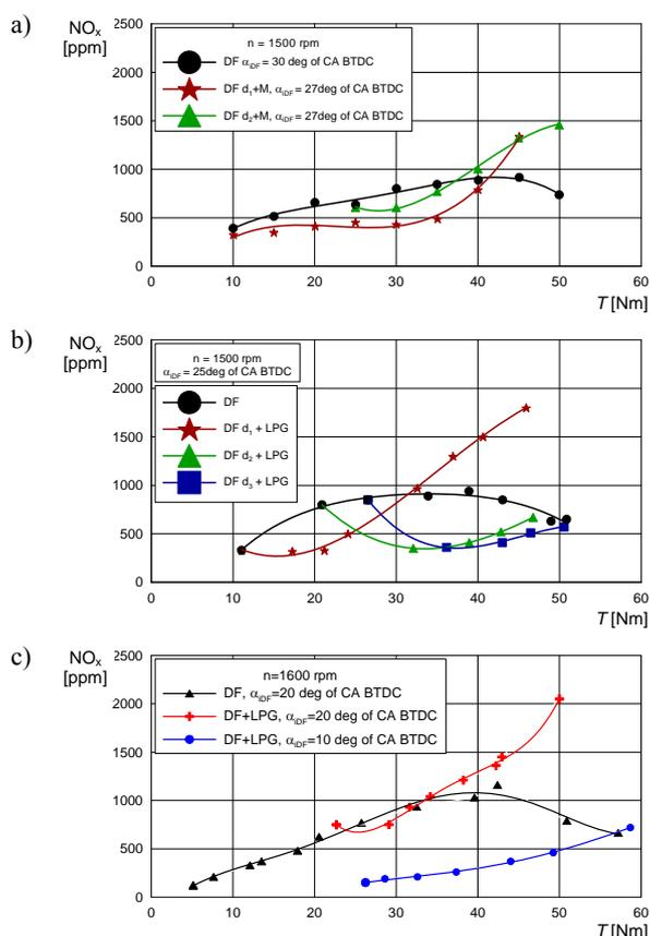
Fig. 5. Comparison of NO<sub>x</sub> emissions for fuelling modes: a), b) and c) (described in chapter 1)
