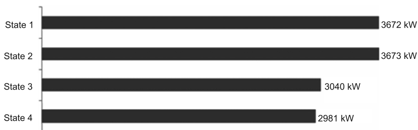
Fig. 7. Active power in different arc work states
