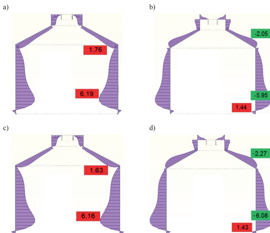
Fig. 10. The distribution of circumferential stresses in composite cross-section: a), b) on the inner and outer surfaces during operation; c), d) on the inner and outer surfaces in the emergency situation
