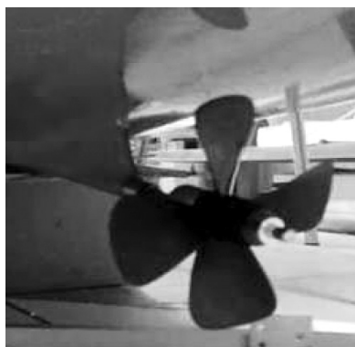
Fig. 5. Propeller, diameter of 9 cm
