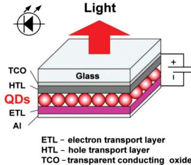
Fig. 5. Schematic picture of a thin film LED with semiconductor nanocrystals [24]
