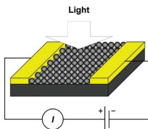
Fig. 6. Schematic picture of a typical NCs-based photodetector [24]
