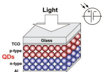
Fig. 7. The schematic solar cell with n- and p- conductivity [24]
