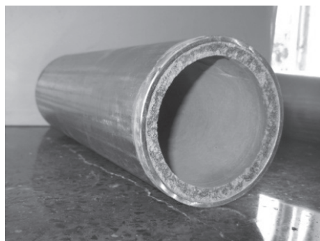
Fig. 2. Steel pipes with internal cement coating (Source: author's photo)
