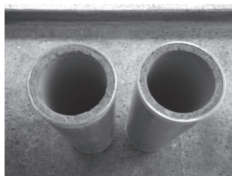
Fig. 2. Steel pipes with internal cement coating (Source: author's photo)
