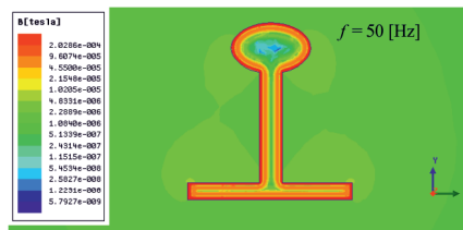
Fig. 8. Distribution of flux density B for f = 50 Hz
