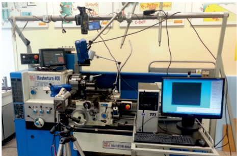
Fig. 3. Research stand for recording phenomena in the cutting zone in turning
