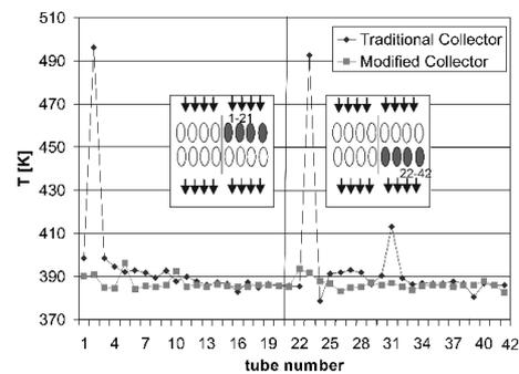
Fig. 17. The bulk temperature distribution in tubes in the second pass of the heat exchanger
