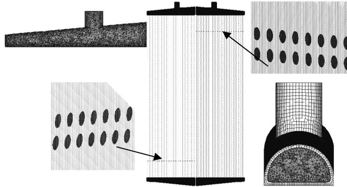
Fig. 6. The high performance heat exchanger divided into finite volumes
