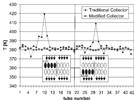
Fig. 16. The bulk temperature distribution in tubes in the first pass of the heat exchanger
