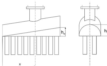
Fig. 5. The geometrical parameters of the modified construction of the collector
