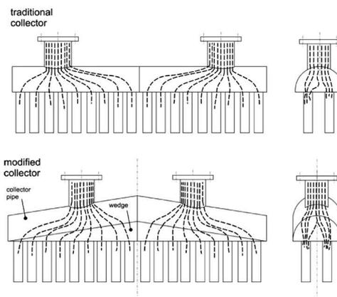
Fig. 3. The traditional and the modified collectors
