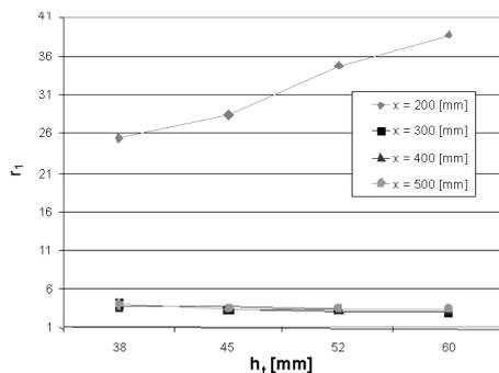
Fig. 8. The values of  $r_1$  as a function of  $x$  and  $h_t$  for  $h_w = 40$  mm
