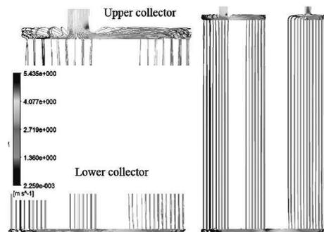
Fig. 7. The flow distribution in high performance heat exchanger with traditional collector
