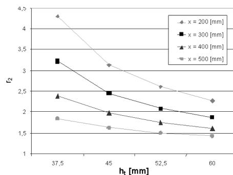
Fig. 11. The values of  $r_2$  as a function of  $x$  and  $h_t$  for  $h_w = 50$  mm
