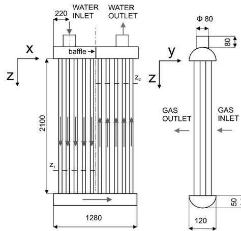
Fig. 4. The scheme of the two-pass high performance heat exchanger
