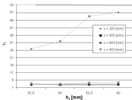
Fig. 10. The values of  $r_1$  as a function of  $x$  and  $h_t$  for  $h_w = 50$  mm
