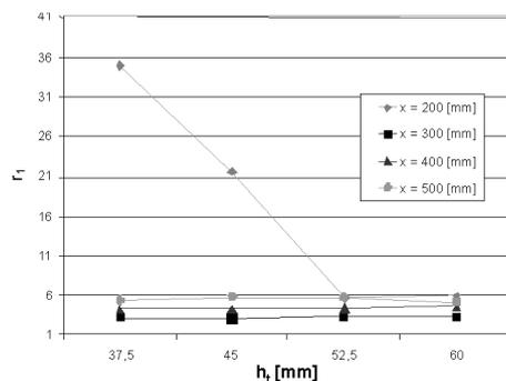
Fig. 14. The values of  $r_1$  as a function of  $x$  and  $h_t$  for  $h_w = 70$  mm
