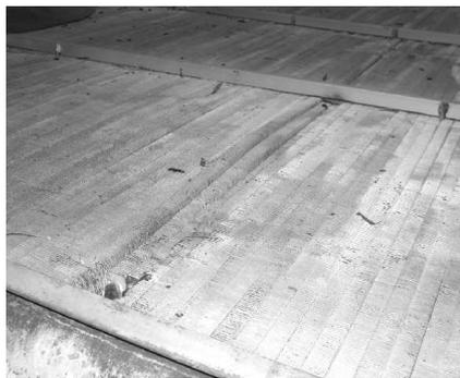
Fig. 2. The buckled tubes of the high performance heat exchanger
