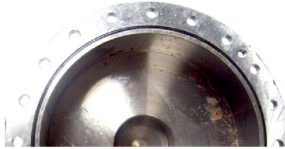
Fig. 9. Corrosion spots inside the dual clutch housing
