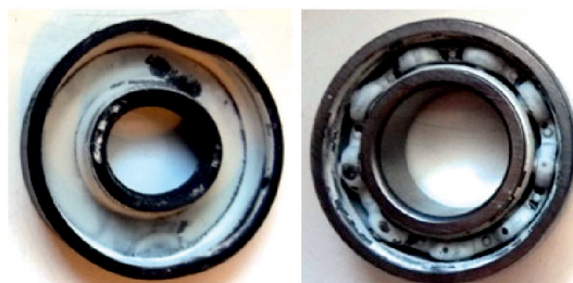
Fig. 5. View of solid particles in the electrorheological fluid in bearings and on the sealing ring inner surfaces
