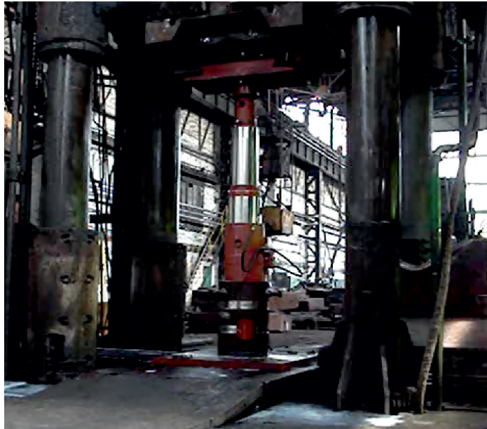
Fig. 2. Tests of actuators in a hydraulic press [2]
