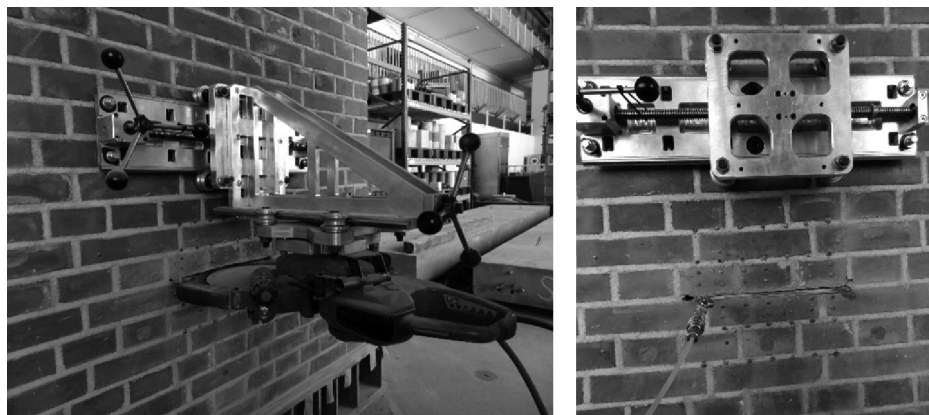
Fig. 3. High precision slot cutting using the RING type circular saw and designer stand (on the left) and view of the wall during the flat jack test (on the right)
