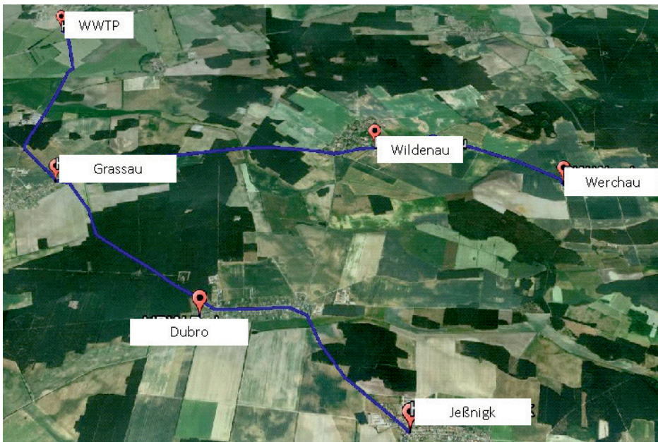
Fig. 1. Scheme of the wet pit pumping station network Grassau, displaying all five wet pit pumping stations and their relative positions to each other
