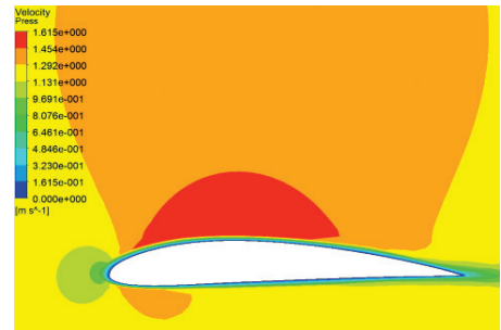
Fig. 7b. NACA 4418: velocity distribution
