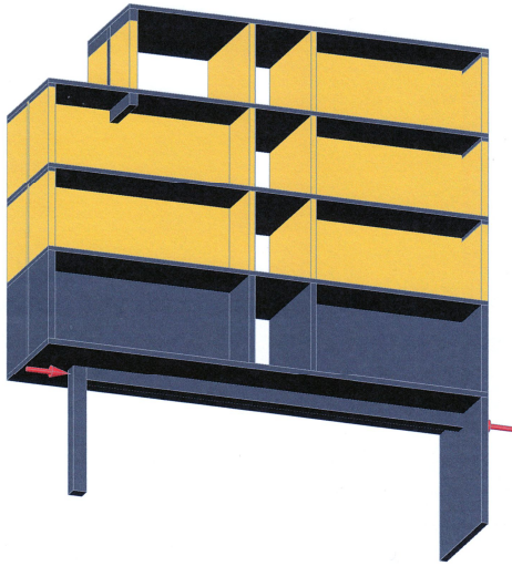
Fig. 4. The scheme of separated support post-tensioned element.
