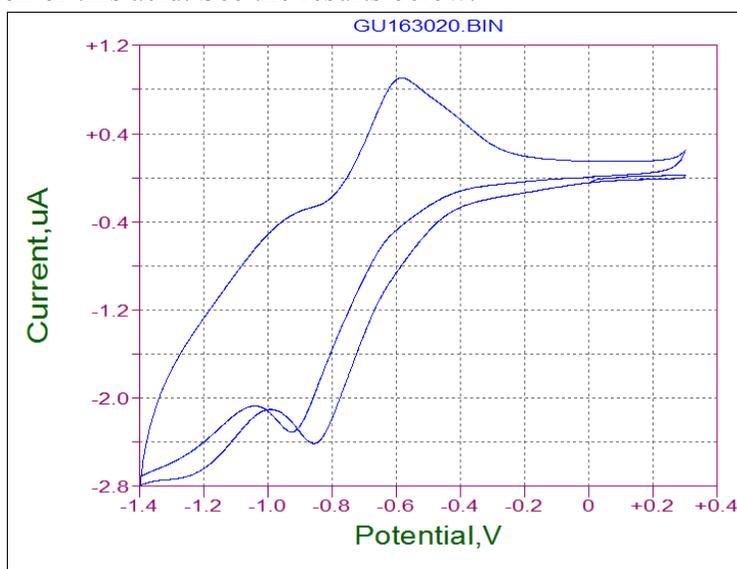
Figure 94. Cyclic voltammograms of citrazinic acid in DMF on Pt electrode.
