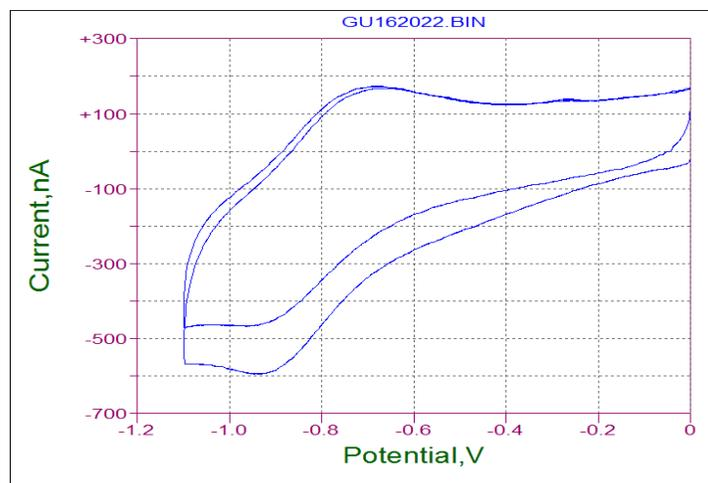
Figure 96. Cyclic voltammograms of polymer in DMF on Pt electrode.
