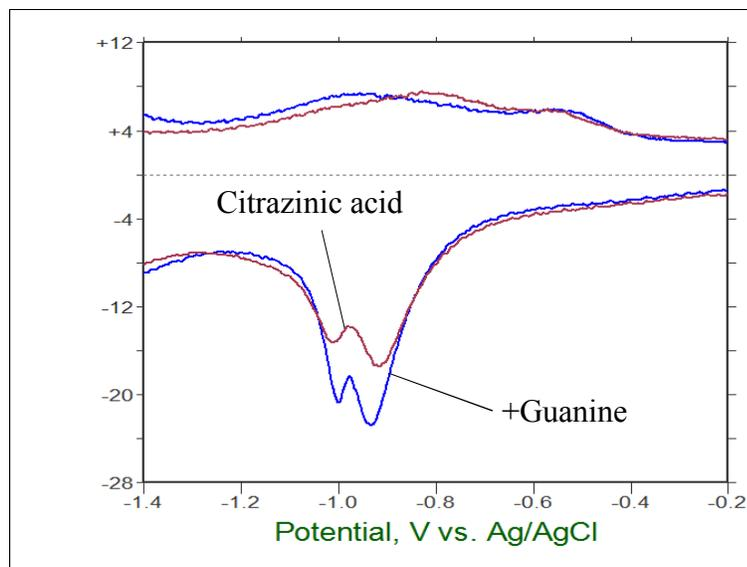
Figure 99. Semiderivatives of voltammograms of citrazinic acid, without and with guanine added in DMF at Pt. Scan rate  $0.02 \text{ V s}^{-1}$ .
