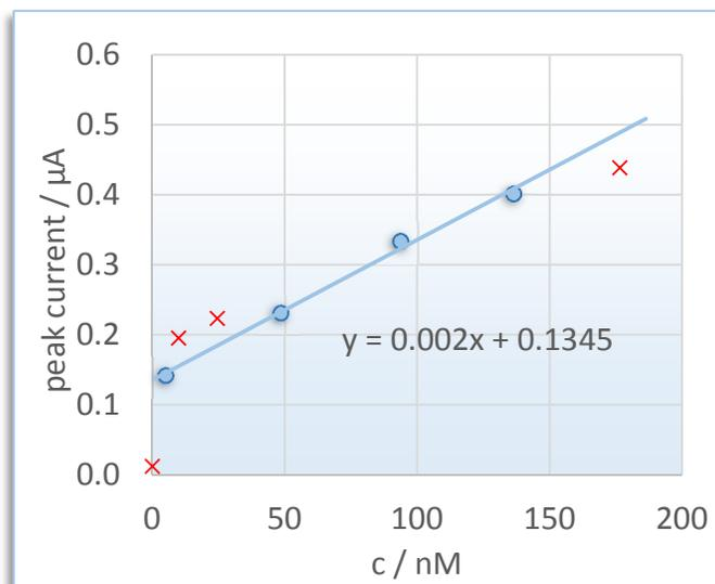
Figure 63. Peak current vs. concentration. Problems at the lowest concentrations. Red crosses denote outliers, not taken for the calculation of the regression equation.
