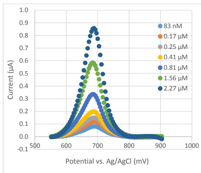
Figure 60. SQWV results. Limit of detection-increasing of current versus guanine concentration.
