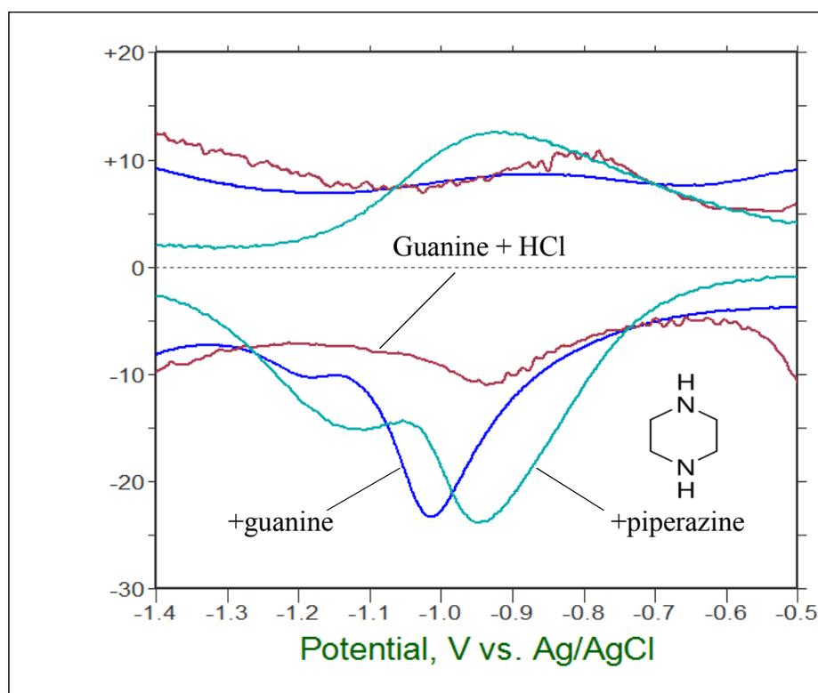
Figure 101. Comparison of semiderivatives of voltammograms of indicated mixtures in DMF at Pt. Scan rate  $0.2 \text{ V s}^{-1}$ .
