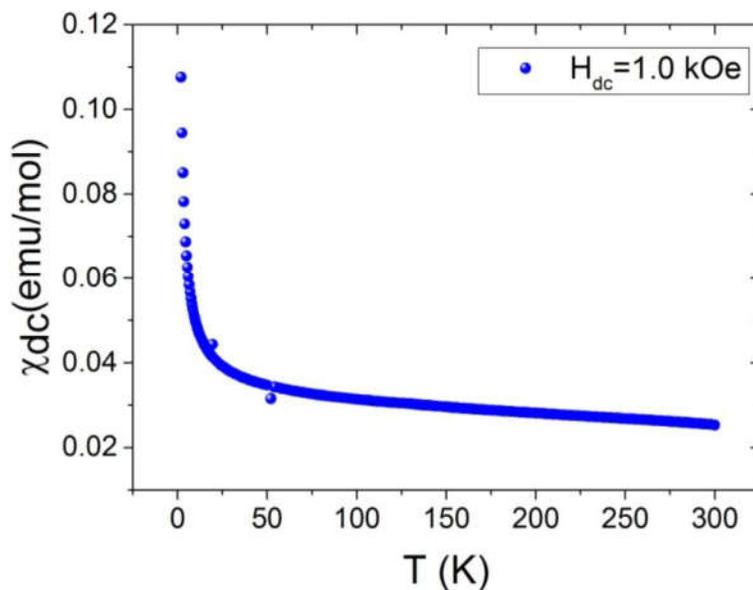
Figure 92. Dc susceptibility as a function of temperature in constant field of 1000 Oe.
