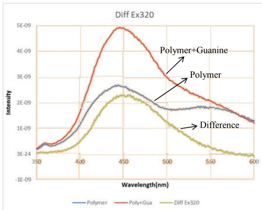
Figure 88. Fluorescence spectra of polymer in the absence and presence of guanine. And the difference between these two spectra at pH 9.
