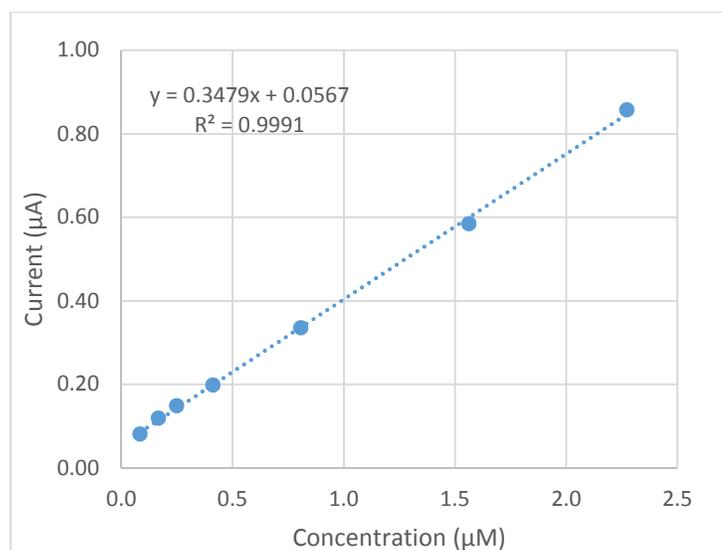
Figure 61. Linear relationship between guanine concentration and current down to 0.08 µM.
