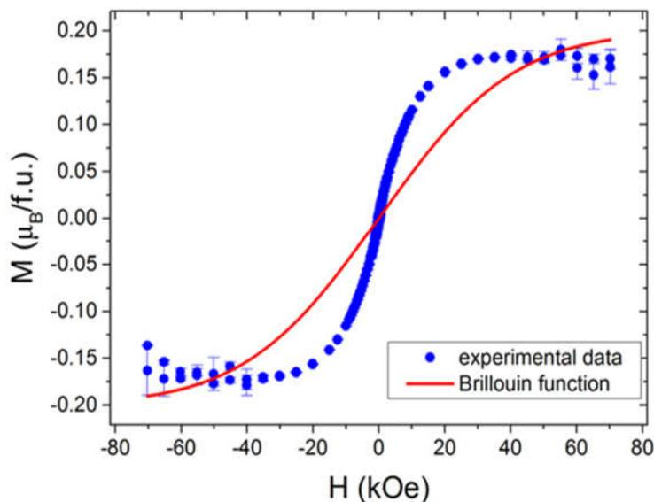
Figure 91. Isothermal magnetization in 2.0K with subtracted diamagnetic contribution (blue circles). The red line represent the Brillouin function for spin 1/2,  $g=2.0$  and with assumption that there is one delocalized electron for each 5 formula unit.
