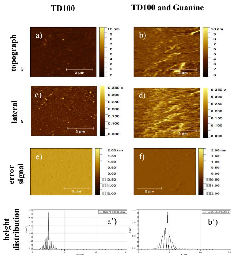
Figure 102. Representative surface topography images of citrazinic acid layer (a) and citrazinic acid admixed with guanine film (b). Lateral force (c, d) and error signal (e, f) images of investigated samples. Additionally, pixel height distributions are presented in (a') and (b').
