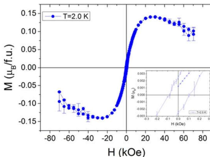
Figure 90. Isothermal magnetization in 2.0 K. Insert points out the value of coercive field of about 90 Oe. The lines are only guides for eyes.
