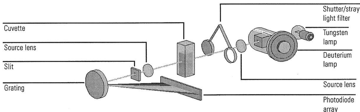
Scheme 8. HP UV-visible Spectroscopy system.
