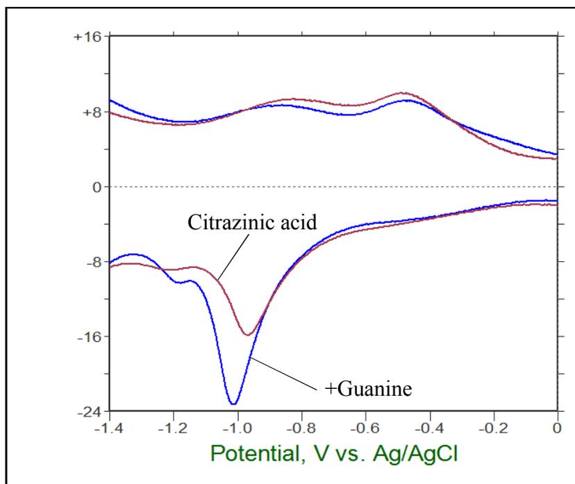
Figure 100. Semiderivatives of voltammograms at a scan rate  $0.2 \text{ V s}^{-1}$ .
