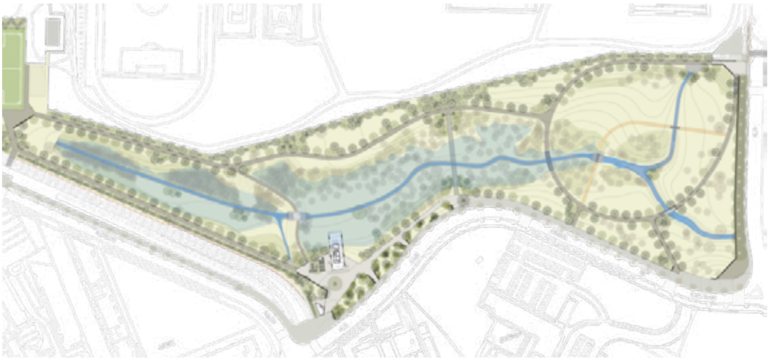
Figure 5. Simulation of the water level at the event of a 100 year storm
