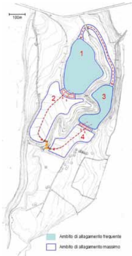
Figure 5. Scenario S1.c: Off-line flood storage reservoirs
