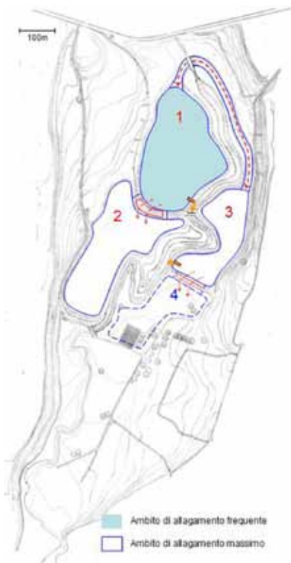
Figure 4. Scenario S1.b: Off-line flood storage reservoirs - Minimizing land transformations
