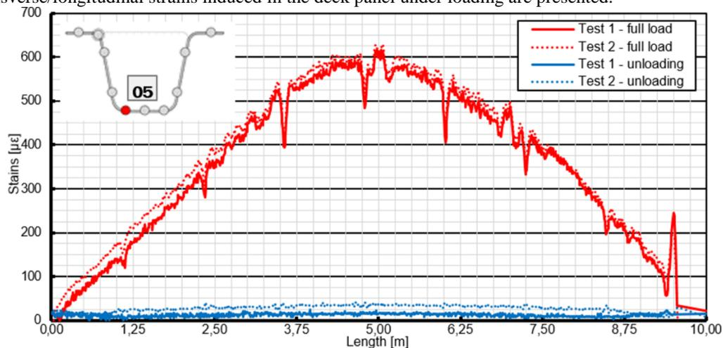
Figure 6: Graph of the strains measured with the DFOS no. 05 – the bottom flange of G1
