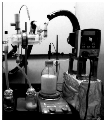
Fig. 4. PFD diagram of the experimental set-up of the decanter (left), picture of the set-up of the continuous separation of a three phase micellar multiphase system (right)
