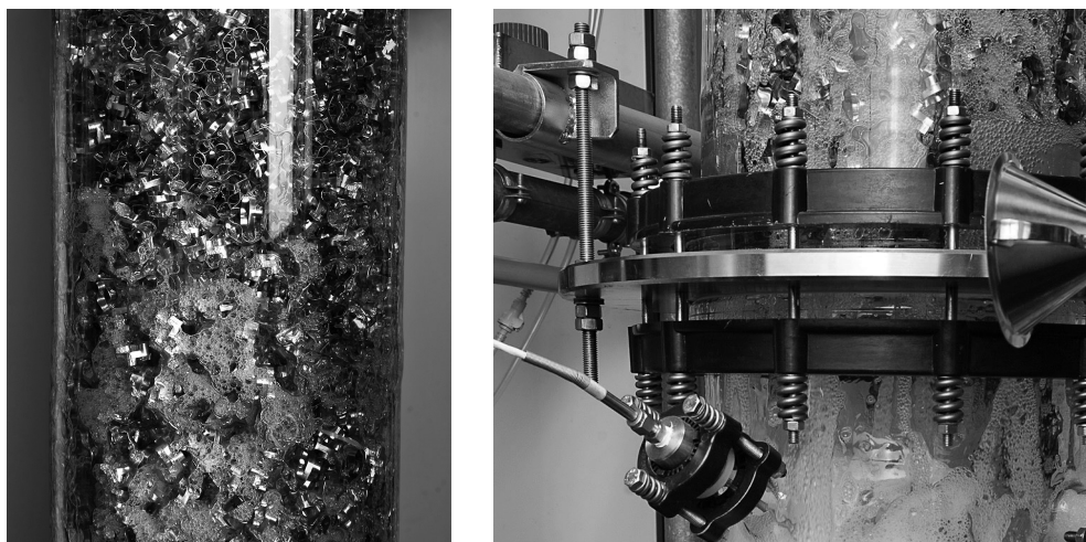
Fig. 1. Foam in random packing McPac #0.75 (left) and foam-flooded column bottom (right) with Triton X-100 30 mg/L at L = 30 \text{ m}^3/\text{m}^2\text{h} and F\text{-factor} = 0.5 \text{ Pa}^{0.5}
